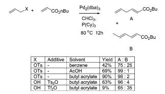
The reaction has been applied to a wide variety of allylic alcohols using the in situ tosylate generation protocol, since many allylic tosylates are difficult to isolate.
